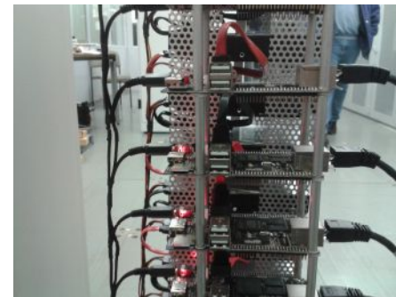
test-cluster with 16 ARM processors and SATA Disks at KIT (SCC)
