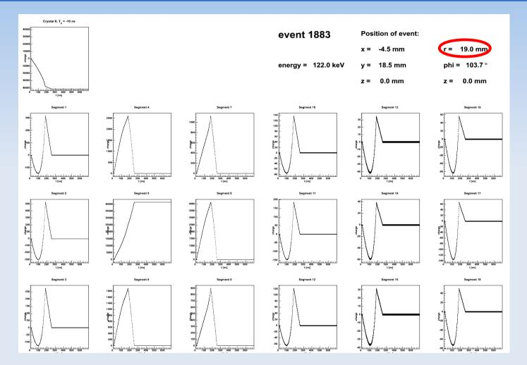
Positive and negative mirror pulses: events at intermediate radii hole and electron both contribute
