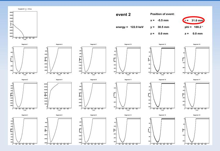
**Negative mirror pulses**: events close to outer segment boundary electron drift towards core dominates pulse shape
