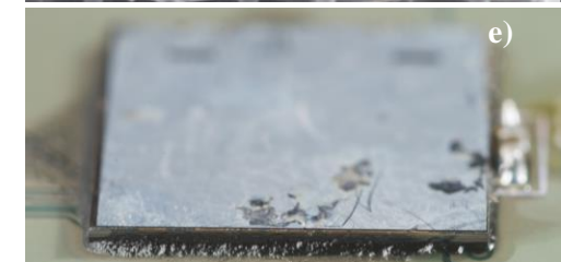
Fig. 1. a) Cartoon of a fully 3D-integrated pixel detector, b) VIPIC1 LTD-bonded on the sensor wafer with back-side bump-bonding pads exposed before wafer dicing, c) VIPIC1 LTD-bonded on the sensor with wire-bonding connections to PCB using traces on the sensor, d) VIPIC1 LTD-bonded to the sensor with bump-bonding Sn-Pb balls deposited on the back, e) VIPIC1 LTD-bonded on the sensor bump-bonded upside down on the precision PCB.
