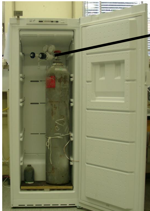
1. CO 2 bottle with pressure regulator pre-cooled to -32°C (saves CO 2 )
