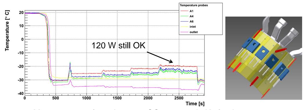
Measurements from the open CO2 system in Karlsruhe, using MPI design in Stainless Steel
