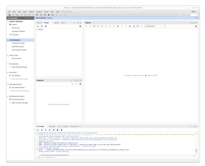
Click on the plus button to add the debouncer IP. You should see our block appearing in the diagram. Since we need three of them, select it, copy and paste it twice (CTRL-C CTRL-P) or right click Copy and right click in an empty place and Paste.
