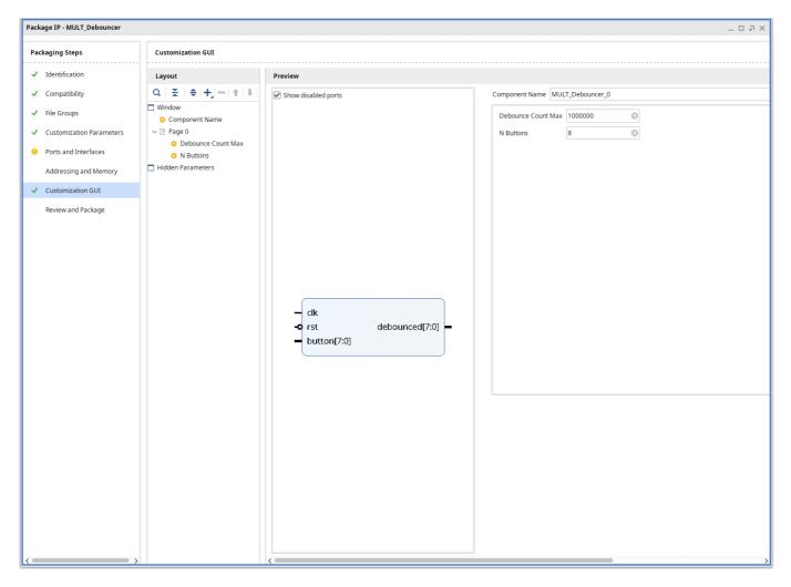
To fix this, go back to the Ports and Interfaces page, and double click on rst, under *Clock and Reset Signals*
