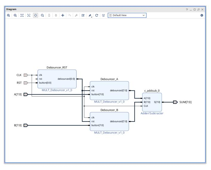
Click on the Validate Design icon You should get a warning that the RST input of the Reset Debouncer block is not connected and will be grounded. That's fine for us. Ignore and click OK. Save the Design (Ctrl-S or the save icon) and close the Block Design context window.
