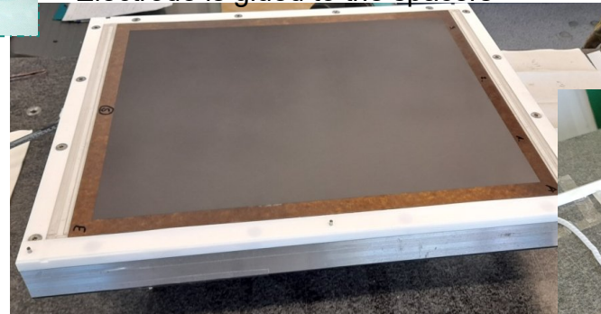
Electrode is glued to the spacers
