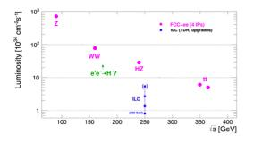
By changing the centre-of-mass energy of the collider the FCC-ee can also be operated as an electroweak and top quark factory.
