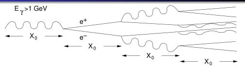
• After a distance  $n \cdot X_0$ :  $2^n$  particles with energy  $E_n \approx \frac{E_{\gamma}}{2^n}$ .
