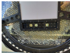
Optical filters in front of certain pixels Blue wavelengths \sim 420 nm
