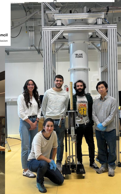
Cryostat with T < 7\text{mK} and B = 12\text{T} installed at MPP in early November
