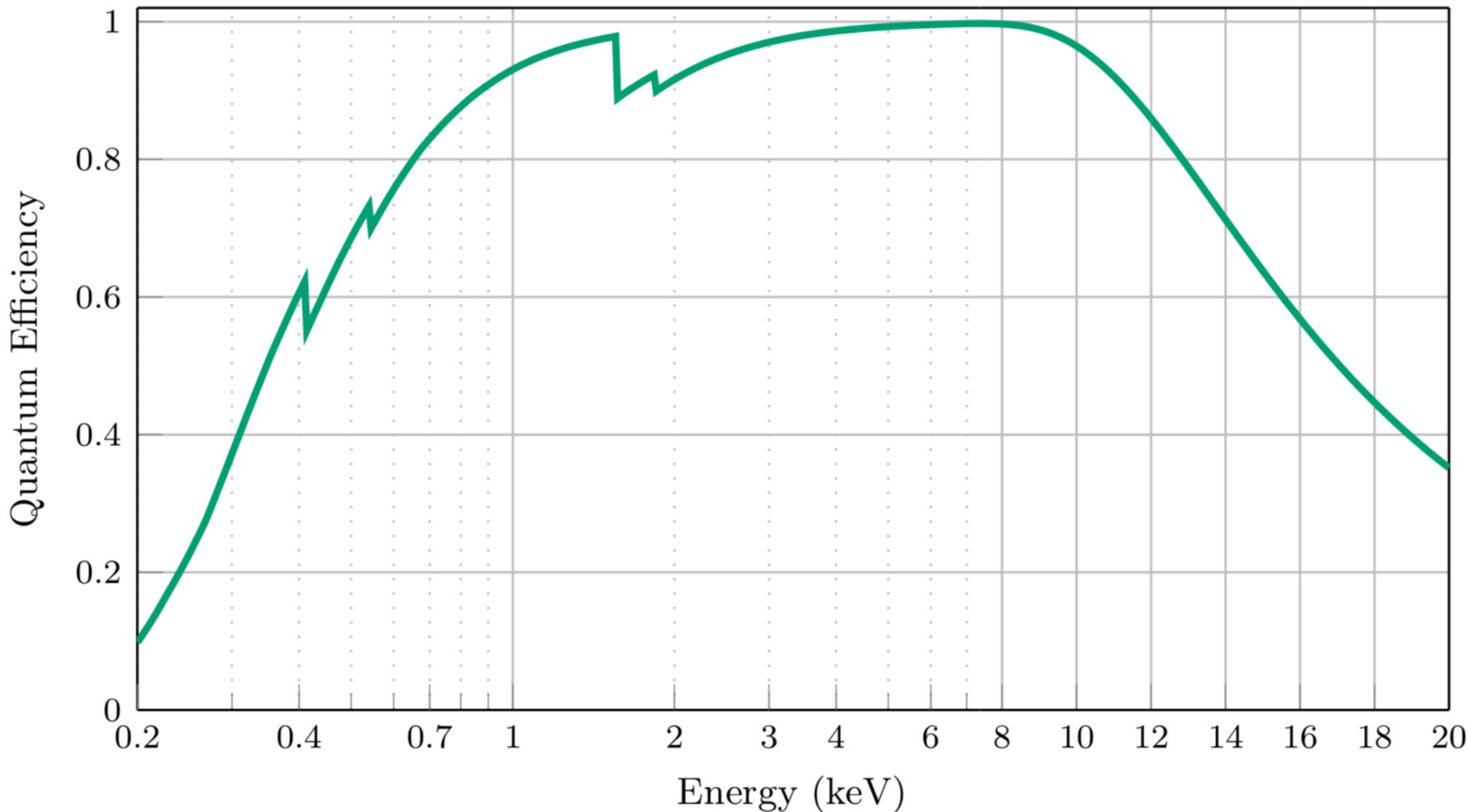
Theoretical QE for a 450  $\mu\text{m}$  thick silicon sensor with a 90 nm aluminium on-chip filter
