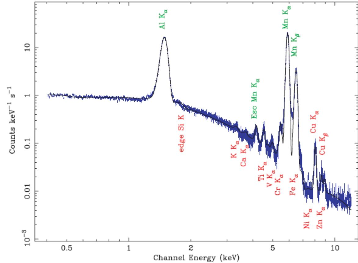
Calibration spectrum with the internal radioactive source
