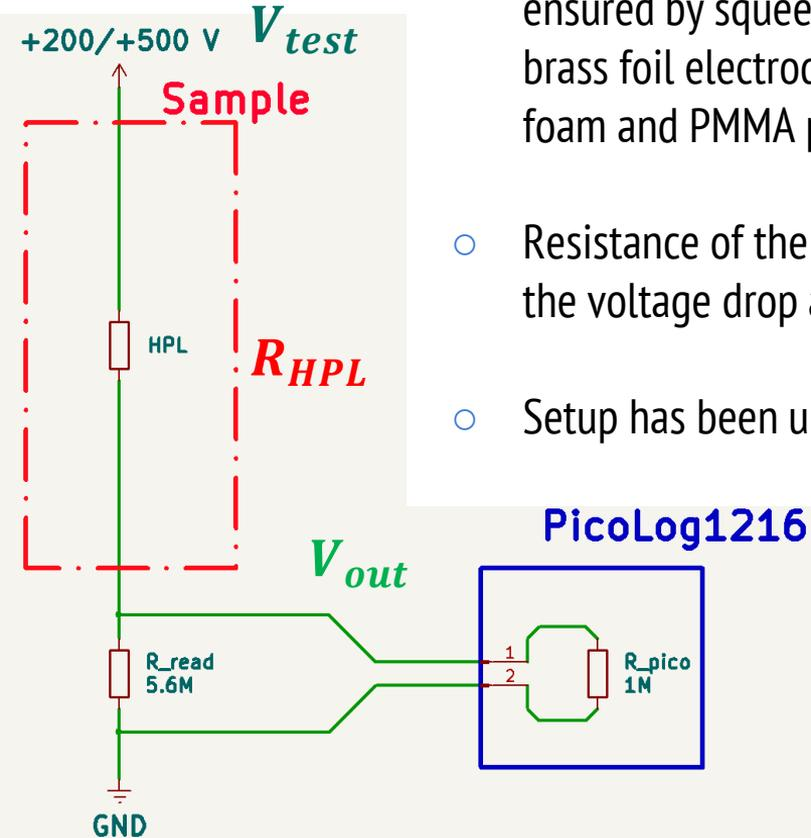
$$R_{HPL} = R_{read} \parallel R_{pico} \left( \frac{V_{test}}{V_{out}} - 1 \right)$$
