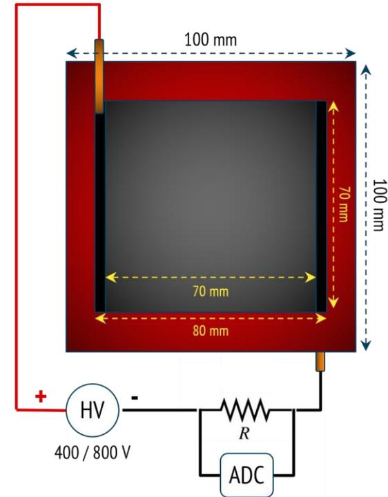
$$R_{tot} = R_{read} \parallel R_{pico} \left( V_{test} / V_{out} - 1 \right)$$
