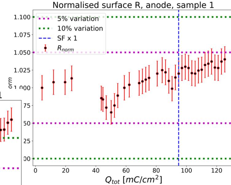
Small variations observed, but within acceptable limits ( $\approx 5\%$  for anode,  $\approx 15\%$  for cathode @ 800 V).
