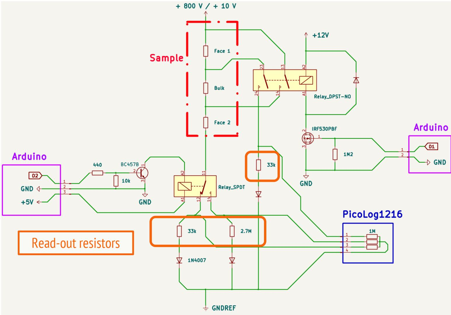
An HV PS provides power to the samples and a reference ground for measurement
