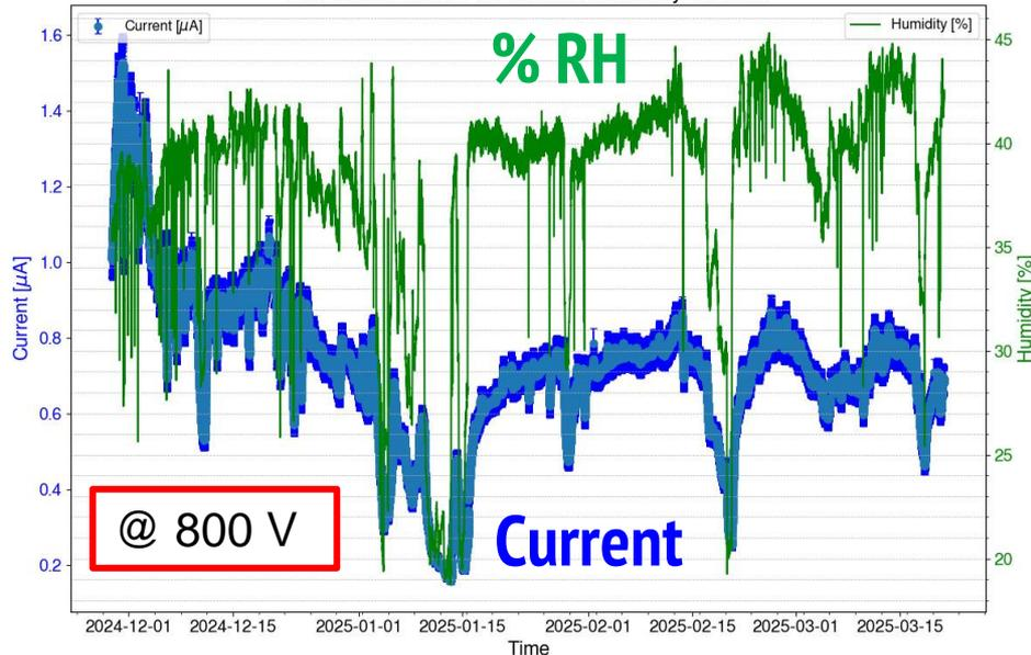
Channel 10: Current vs. Time and Humidity vs. Time
