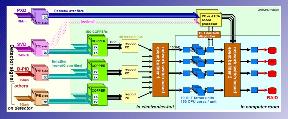
\* Track parameters are obtained in High Level Trigger and sent to PXD readout processor.
