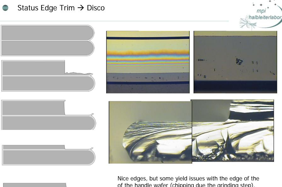
of the handle wafer (chipping due the grinding step). Needs still some improvement ..
