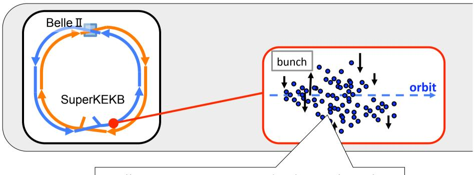
oscillation motion perpendicular to the orbit ("betatron oscillation")
