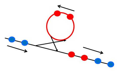
Inject alternatively (50 Hz), but extract from damping ring in phase (same Linac pulse)
