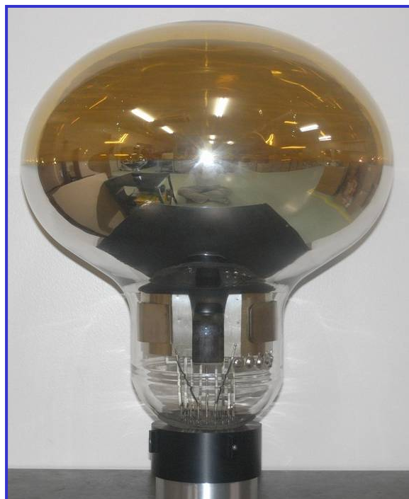
R11780 / 12-inch PMT for Neutrino Experiment
