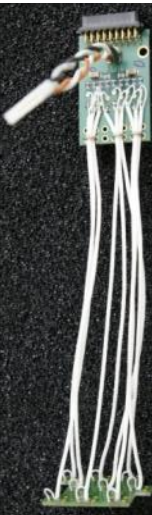
Completed sensor plane
