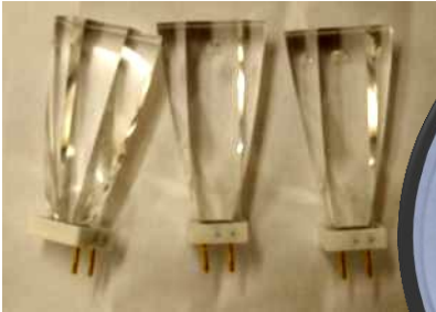
1) MPPCs – cone gluing
