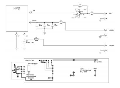
Use of a Hybrid Photo Detector (HPD) in the MAGIC micro power LIDAR system
