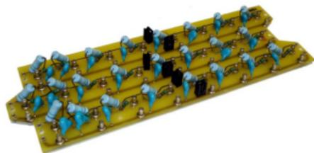
Prototype of new radiation hard active front-end cards
