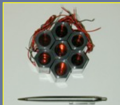
GaAsP HPD (MPI & Hamamatsu): 50% PDE
