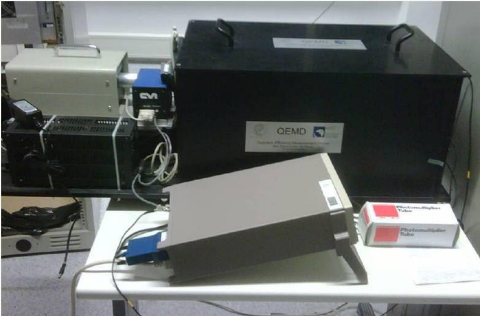
Quantum Efficiency Measurement Device for PMTs
