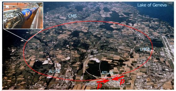
The Large Hadron Collider is a 27 km long collider ring housed in a tunnel 100 m underground near Geneva.
