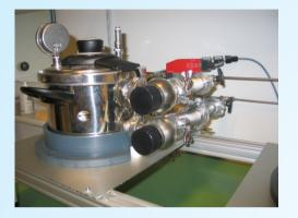
Serially produced detectors are to reveal whether they functions within predefined parameters. Short tests [order of one day]
