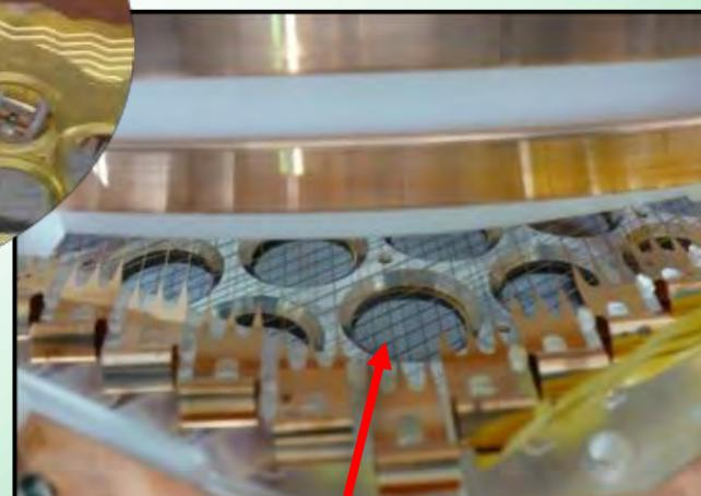
Charge detection wires
