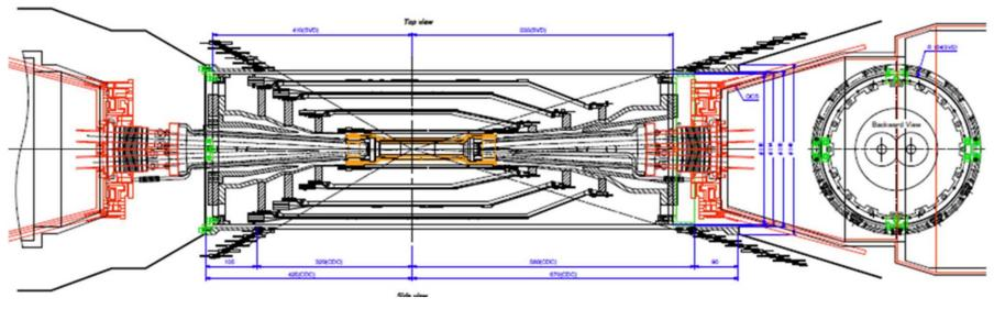
Space at Forward QCS too tight for manual vacuum connection Baseline installation: mount VXD on QCS and move together through CDC
