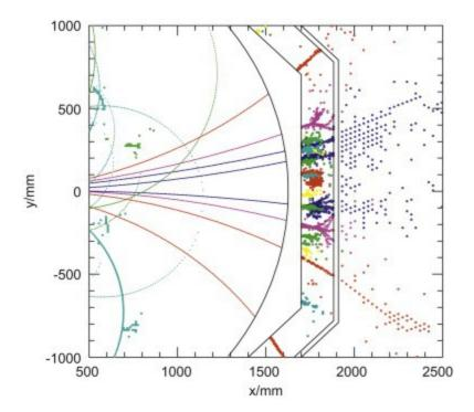
**Particle Flow:** highly granular calorimetry inside a large 3.5-5 Tesla solenoid allows to follow every single visible particle produced in the collisions from the cradle to the grave  $\rightarrow$  best possible estimate of the jet energy:  $\Delta E/E \sim 3-5\%$
