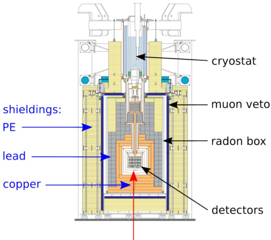
new: inner neutron shielding - 5 cm PE
