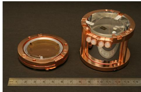
CRESST-II module with a CaWO<sub>4</sub> target
