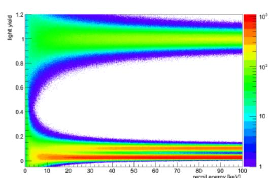
LY scatterplot for PbWO<sub>4</sub> with an uniform energy distribution
