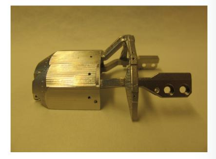
The finally cooling block for thermal tests, a 3D metal print (non magnetic stainless steel)
