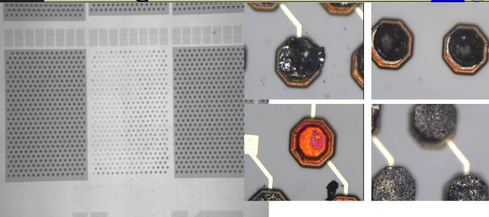
Not all the balls were properly soldered on substrate pads. Nevertheless, no solder paste spread out during chip removal in any of the chips we removed
