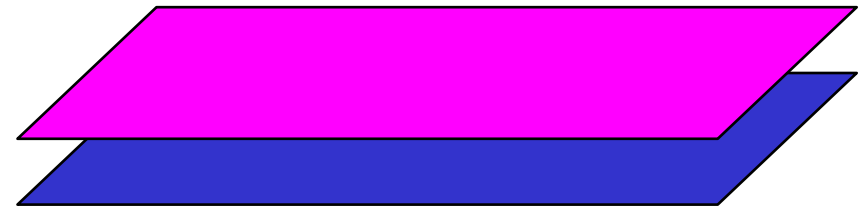
Layer Alu1 + layer Alu2 (also called Flat, worst case → no possibilities for stress relief)
