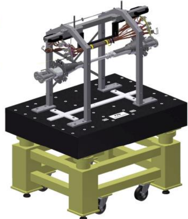
Mounting tool for PXD connection to the beam pipe
