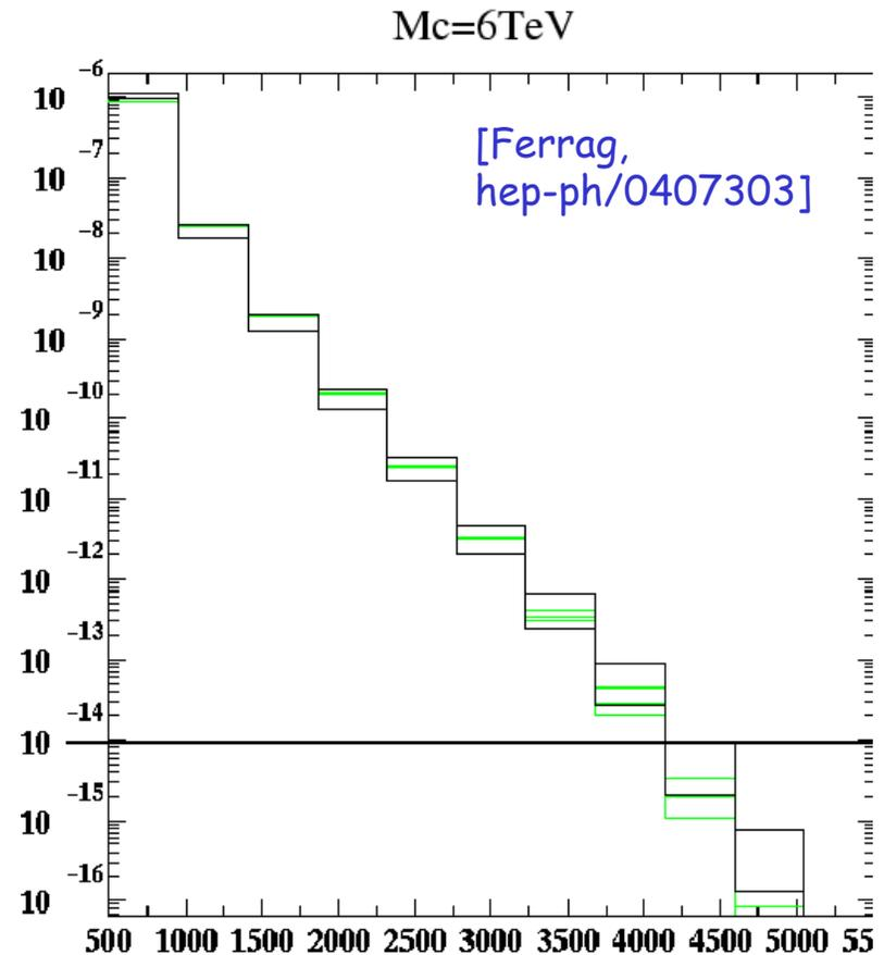
... in this example, high  $x$  PDF uncertainties reduce sensitivity to compactification scales from 6 TeV to 2 TeV for 2 XDs
