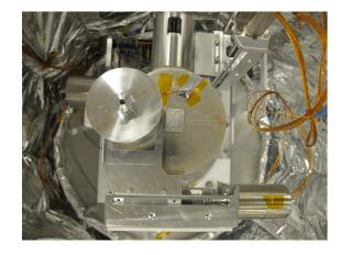
► Collimators slide in groves of infrared shield
