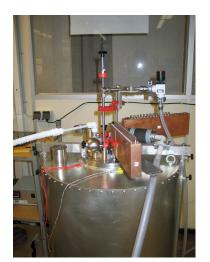
► Test-stand Gerdalinchen-II: Simultaneous operation of up to three segmented detectors in LAr or  $LN_2$
