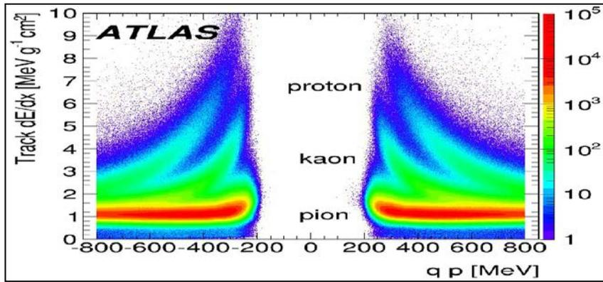
The truncated mean for the energy loss per track as a function of signed momentum for tracks.
