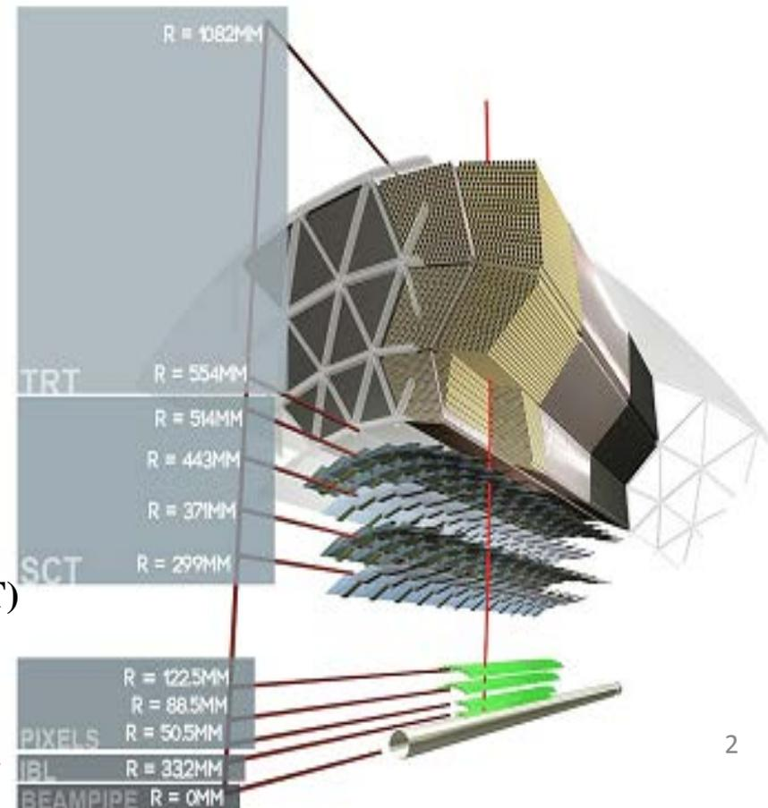
**ATLAS Inner Detector (ID) main tracking device:**
