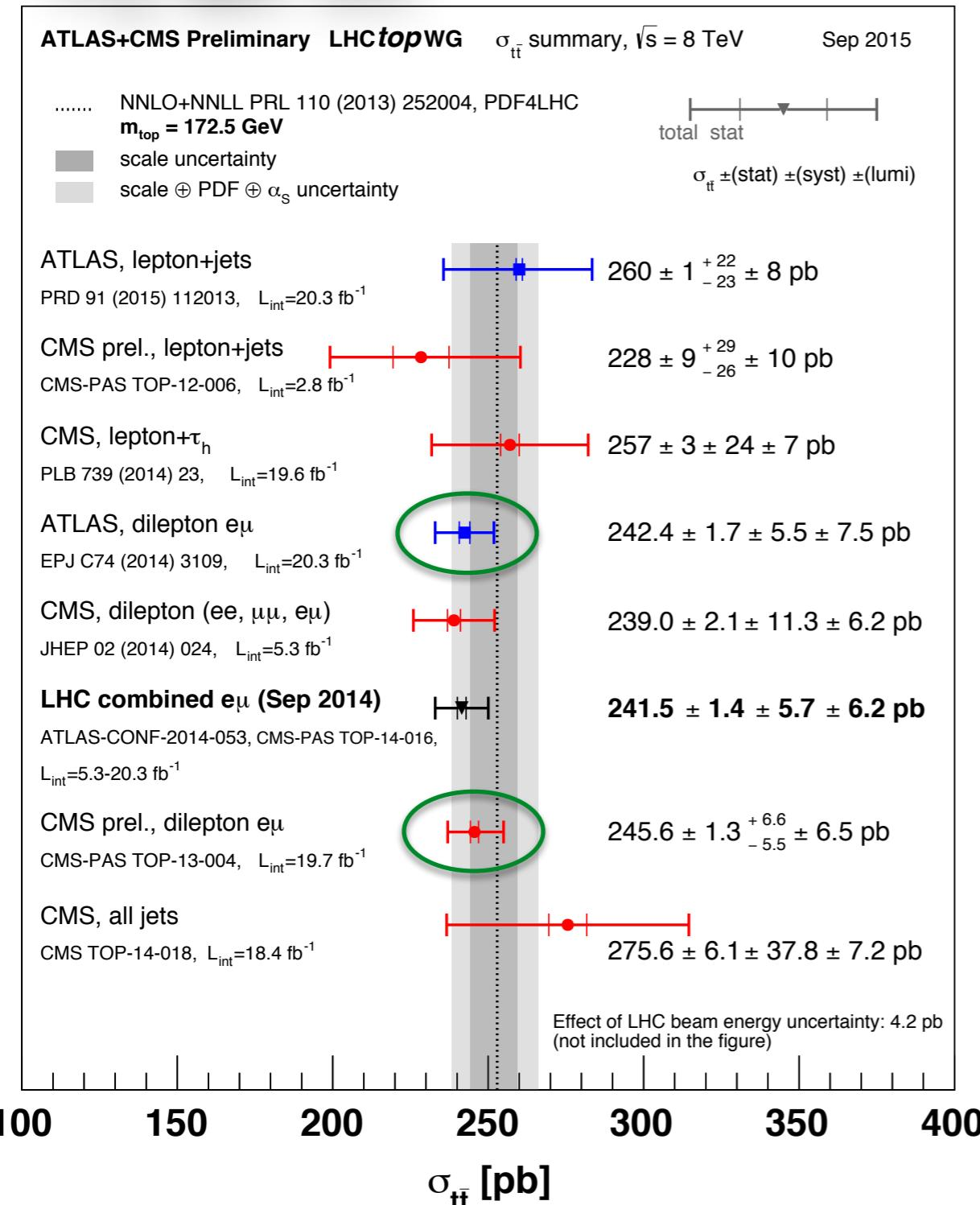
The ATLAS and CMS collaborations have measured the total inclusive cross sections for top pair production at 7, 8 and 13 TeV
