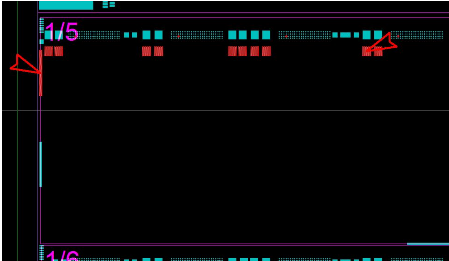
Shorts among drain lines and source pads.
