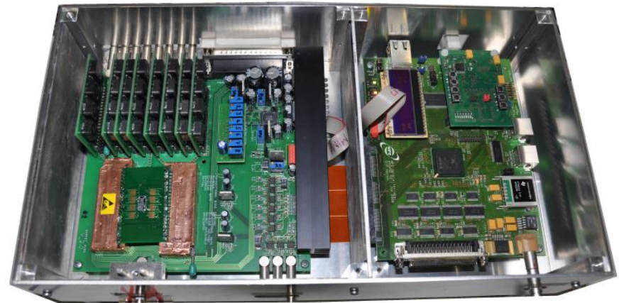
Figure 4.2: Plan view of the mini-matrix box with the main board located on the left side
