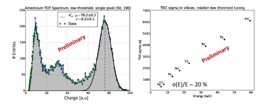
→ FE-I4 (ATLAS-IBL): Fast, adequate energy resolution and minimizes system related problems (radiation hardness and long cables)
