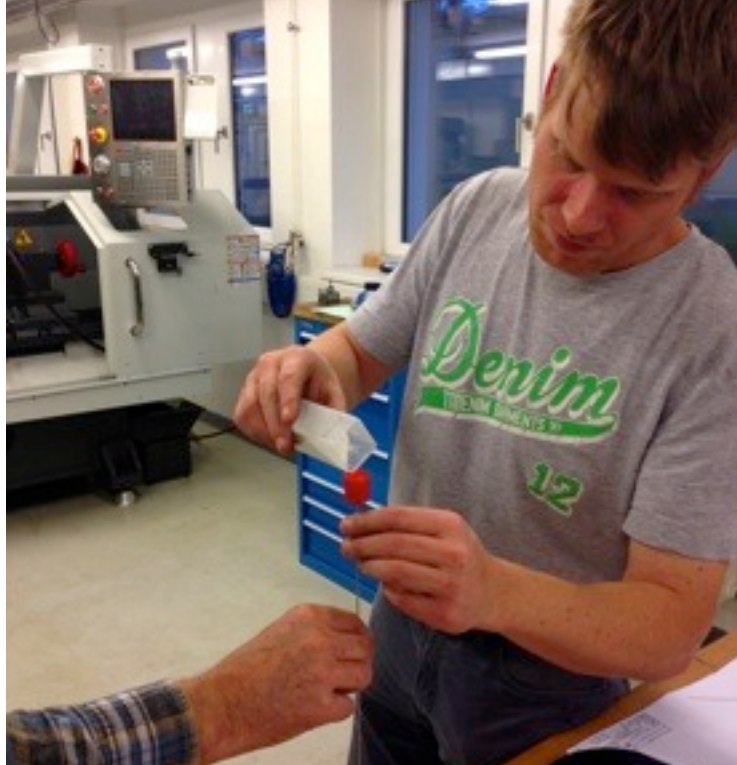
Filling pipe with sand
