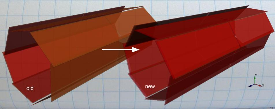
15°; shift -= 0.686 mm; radius += 0.17 mm; DSSD length += 4.86 mm;
