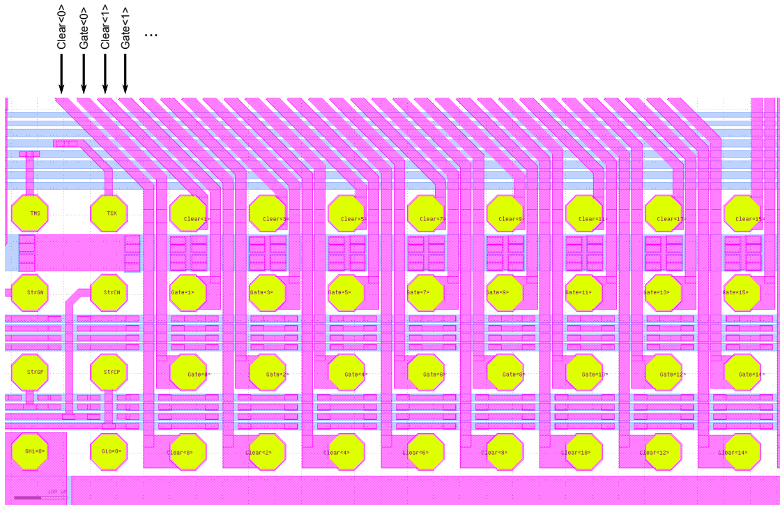
(b) Switcher footprint on the substrate of the half ladder. Both Clear and Gate lines are numbered ascending from left to right.
