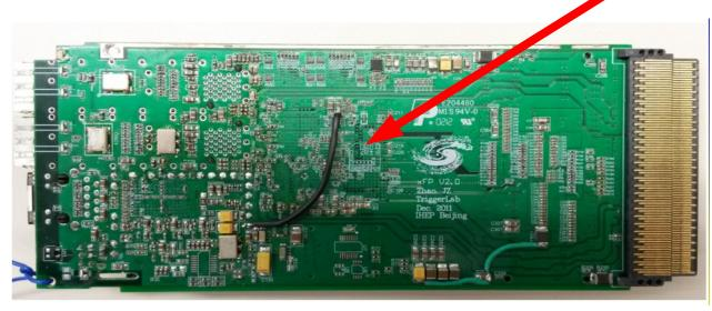
before hotfix: measured voltage on +1V directly below FPGA (C235): 917 mV (confirmed by JTAG measurement)
