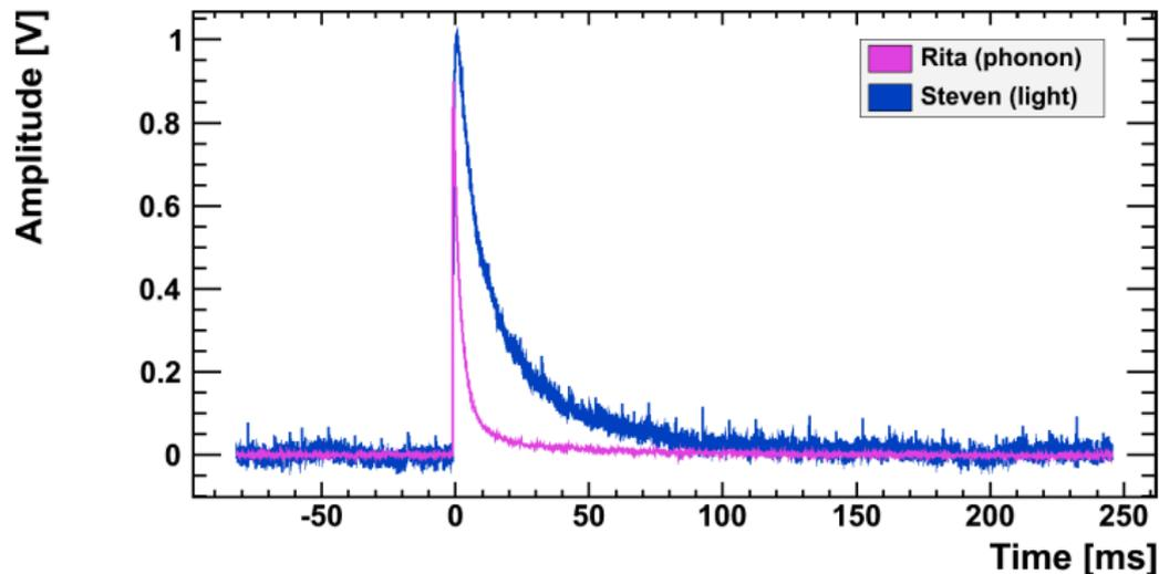
When a particle event occurs most of the energy is converted into phonons (phonon channel). The part converted into photons is measured by the light detector (light channel). Pulses amplitudes are proportional to the respective deposited energies.
