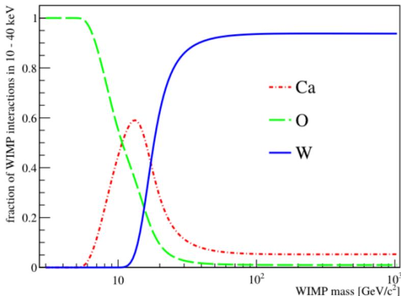
Because of multi-target absorbers, WIMPs are expected to interact differently with different nuclei
