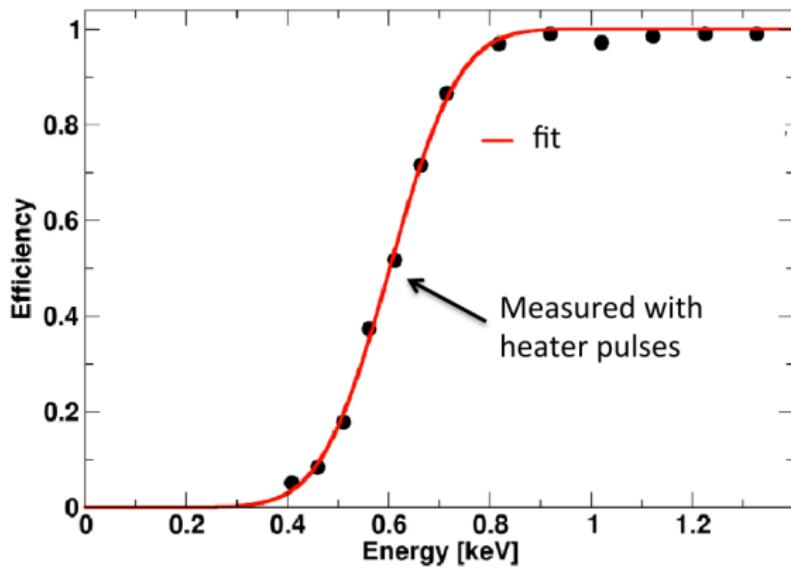
extremely low trigger threshold of  $E_{th} \sim 603$  eV
