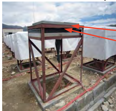
Lead plate (80 cm X 50 cm X 7 rl) Iron plate (1 m X 1 m X 1 rl)
