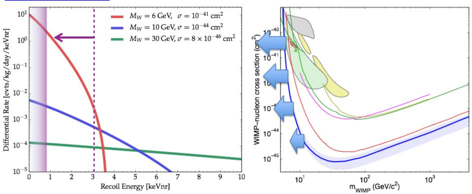
Decreasing this response cutoff from 3 keV to < 1 keV provides access to a factor of 8000 more signal at M = 6 GeV
