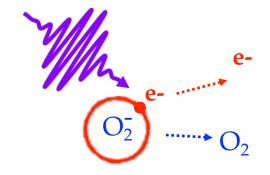
A Xe scintillation photon (7 eV) can eject an electron from the surface of a metal (i.e. one of the electrodes)
